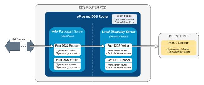
In addition to the two mentioned deployments, two K8s services are required in order to direct dataflow to each of the pods. A LoadBalancer will forward messages reaching the cluster to the WAN participant of the cloud router, and a ClusterIP service will be in charge of delivering messages from the local DS to the listener pod. Following are the settings needed to launch these services in K8s:
