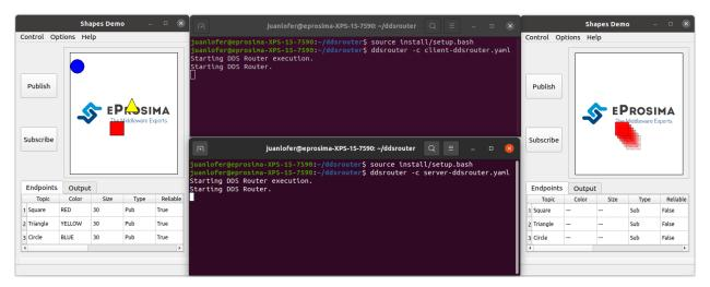
DDS Router supports the dynamic addition/deletion of topics at runtime (see *Reload Topics*). Let us test this feature by adding the circle topic to the allowlist of both routers. Also, by removing the square topic (removing this topic from one of the routers' allowlist will suffice) the square data should stop reaching the subscriber. Alternatively, the square topic may be added to the blocklist, achieving the same effect. See *Topic Filtering* for more details on allowlisting.
