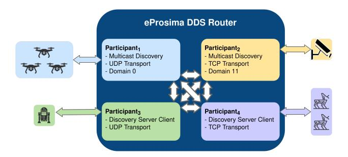
DDS node, publishing and subscribing in the shared DDS topics. This allows to create a non limited and highly scalable decentralized and distributed DDS network.
